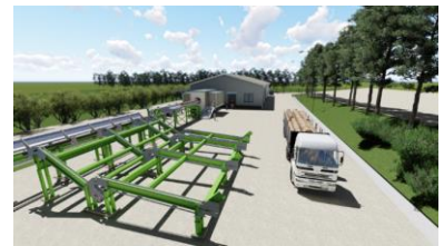
CT LOG SOLUTION X-RAY COMPUTER TOMOGRAPHY FOR DEFECT DETECTION AND QUALITY EVALUATION ON LOGS
