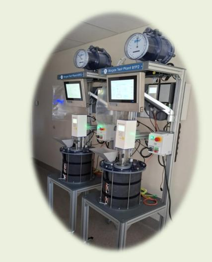
Research stand for aerobic and anaerobic processing of plant biomass and organic waste. The stand is designed to study, model and demonstrate the processes of aerobic and anaerobic processing of plant biomass and organic waste. Research on the biodegradation of biomass and organic waste is necessary for evaluating the potential of biogas and biomethane production, the efficiency of composting processes and the quality of the resulting products.
